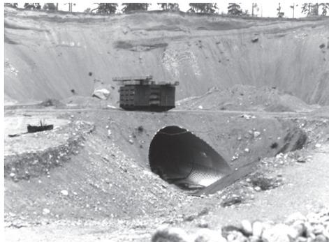
Figure 1. Enköping pipe arch, loading to failure test
