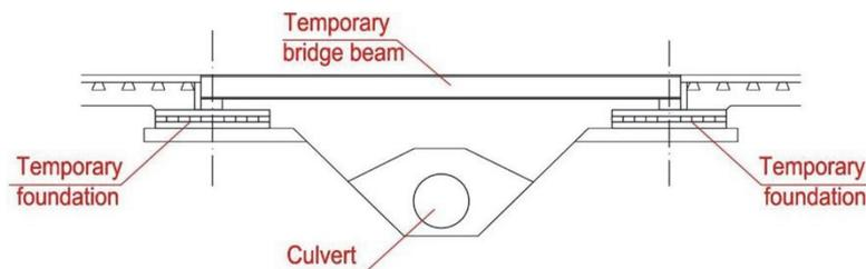
Figure 4. Longitudinal section of temporary bridge beams
