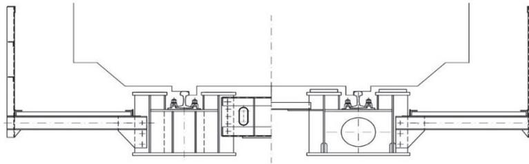
Figure 3. Cross section of temporary bridge beams
