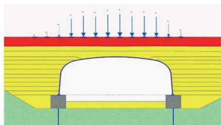
Figure 7. Numerical model of the structure
