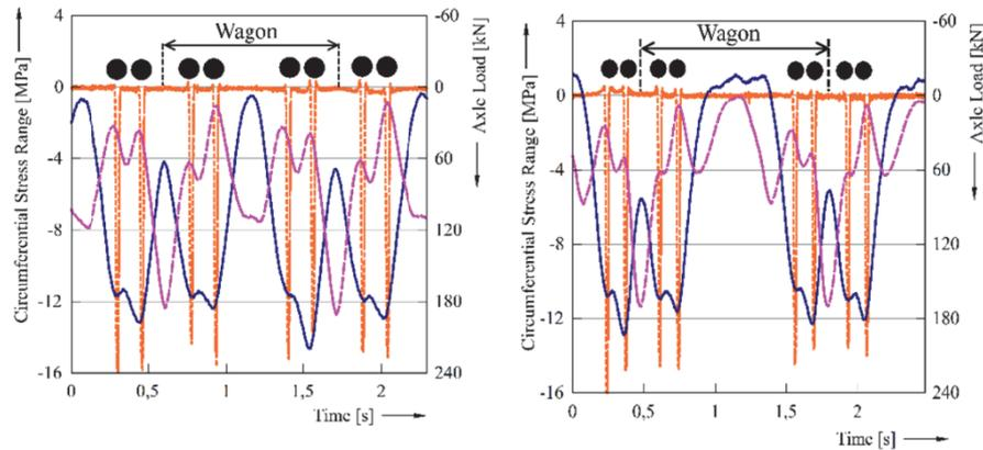
Fig. 3. Typical stress range patterns on the top plate as a group of bogies crosses the bridge. a) Bogie pairs closer together and b) Bogie pairs further apart. [2]
