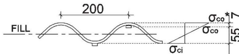
Fig. 2. Cross section of the culvert plate and stress distribution and locations of strain gauges. [2]
