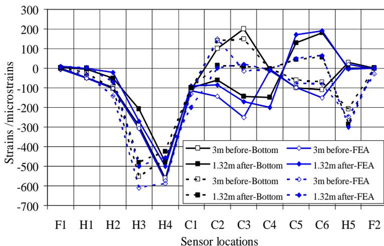
Figure 5. Comparison of the FEA results with top and bottom sensors measurements at different sensor locations for cover depth 0.45 m
