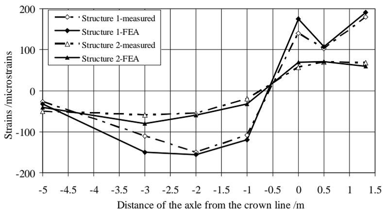
Figure 4. Comparison of the FEA results with bottom sensors measurements at C6 due to different truck positions for 14m-span Structures 1 and 2 with cover depth 0.45 m
