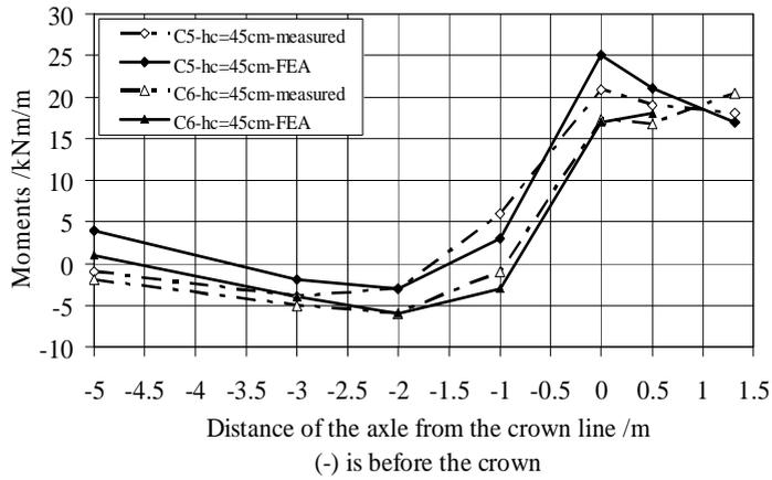
Figure 10. Comparison of the bending moments obtained from FE analyses with measurements at C5 and C6 caused by various truck positions for the depth of 0.45m
