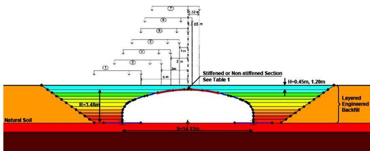
Figure 1. Cross-sectional geometry of the box culvert and the truck positions where the truck approaches the bridge backwards
