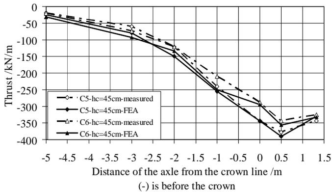
Figure 7. Comparison of the FEA results with measurements at C5 and C6 due to different truck positions for 14m-span Structures 1 and 2 with cover depth 0.45m
