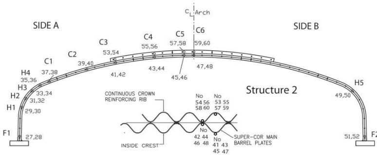
Figure 3. Numbers, locations, and names of the sensors of the 14m-span culvert with crown ribs (Bayoglu Flener, 2010)
