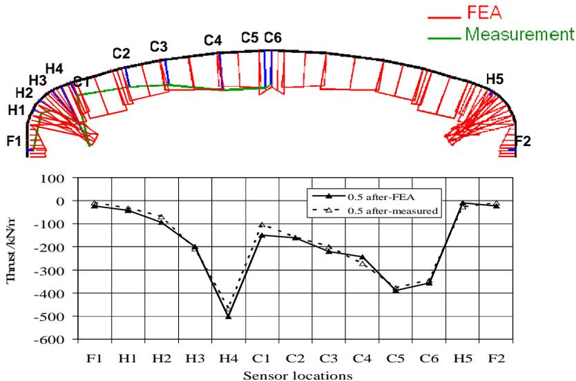
Figure 8. Comparison of the thrust results at different sensor locations for Structure 1 with cover depth 0.45m; not to scale (measurement values from Bayoglu Flener, 2010)
