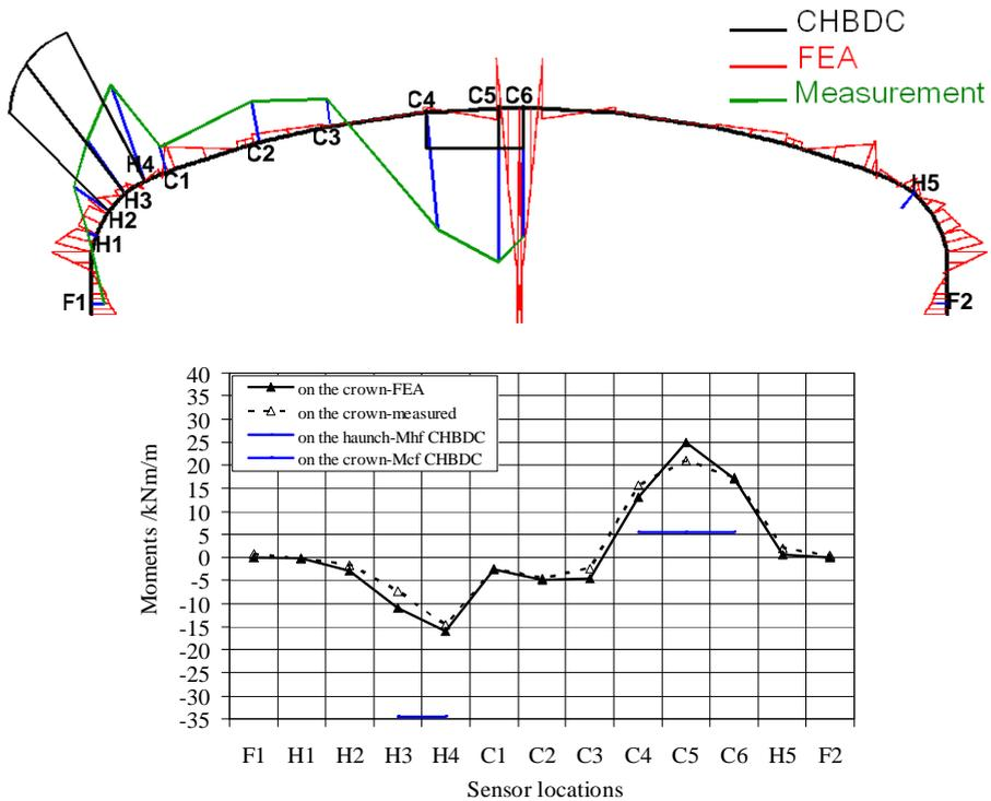
Figure 11. Comparison of bending moments at different sensor locations for Structure 1 with cover depth of 0.45m; not to scale (measurement values from Bayoglu Flener, 2010)
