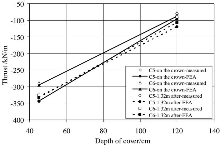
Figure 9. Thrusts at C5 and C6 for Structure 1 with cover depth 0.45m and 1.20m; for truck positions on the crown and 1.32m after crown CL
