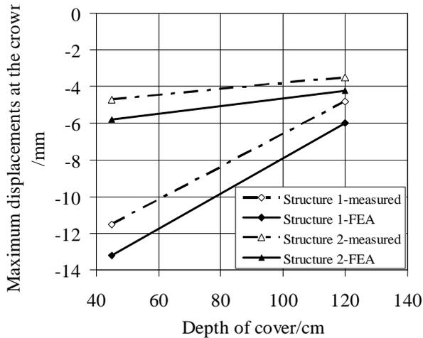
Figure 6. Maximum displacements of the crown during truck loading tests for Structures 1 and 2; negative values indicates downward displacements
