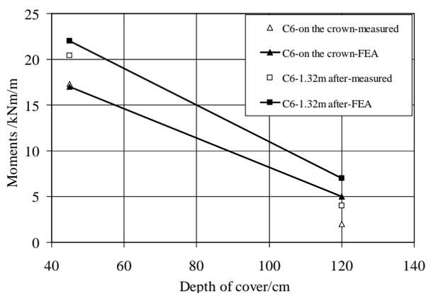
Figure 12. Moments at C6 for Structure 1 with cover depth 0.45 m and 1.20 m; for truck positions on the crown and 1.32 m after crown CL
