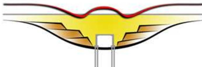
Figure 1. Original design scheme with precast reinforced concrete portal
