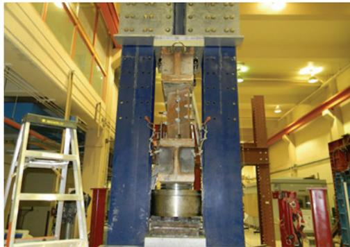
Figure 4. Ultra-Cor Compression Test (Dr. John Newhook, Philip Vickers, 2011b, p. 1)
