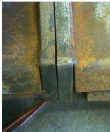
Figure 7. Flange Connection Gap after Testing
