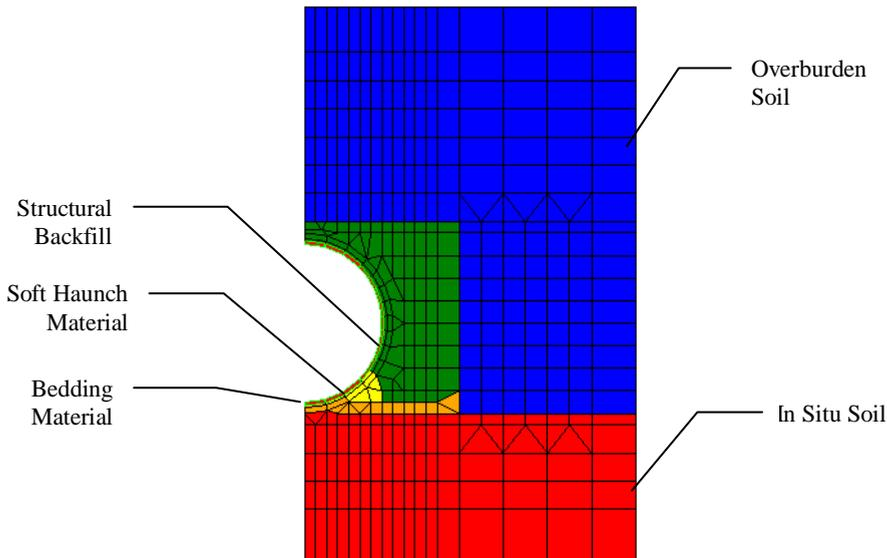
Figure 6 CANDE soil zones for an embankment installation.
