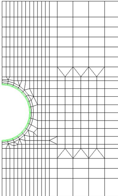
Figure 5 CANDE FEM mesh of the 2.13 m pipe
