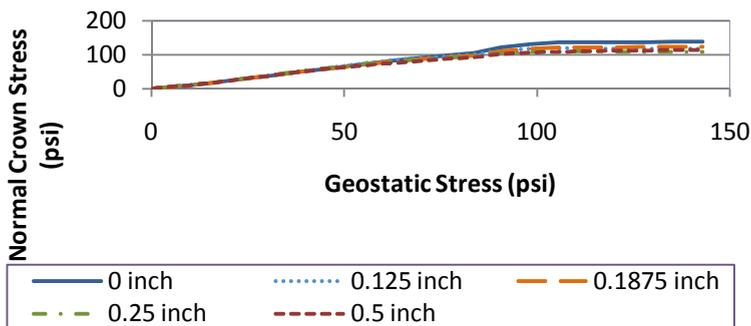
Figure 7 Vertical crown soil pressure versus applied stress for five slotted joint lengths
