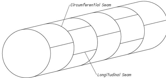
Figure 1 Structural plate pipe showing typical seam configuration
