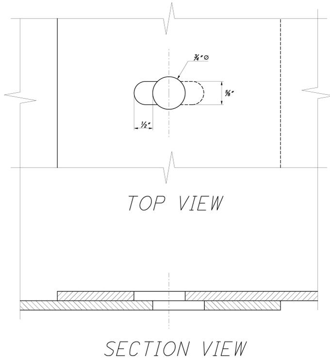
Figure 2 Typical slotted joint configuration
