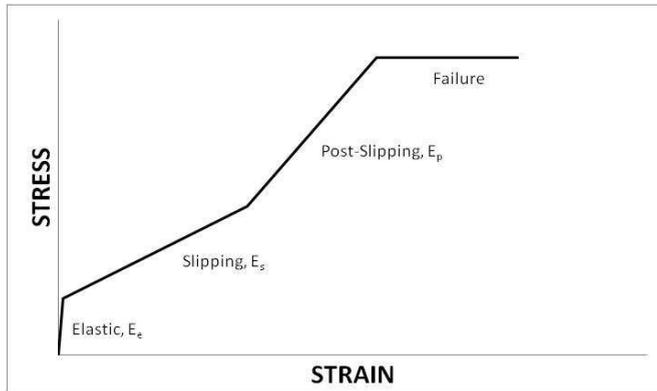
Figure 4 Theoretical model of slotted joint behavior [2]
