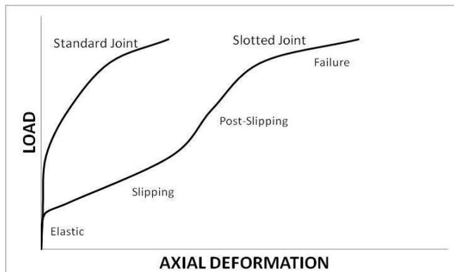
Figure 3 Typical slotted joint behaviour [2]
