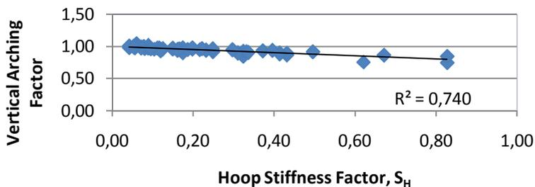
Figure 9 Vertical arching factor versus pipe soil ring stiffness
