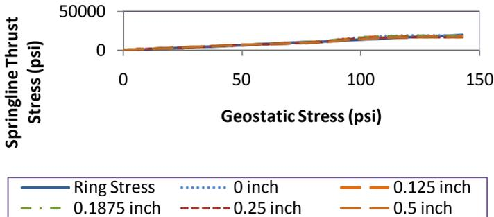
Figure 8 Springline thrust stress versus geostatic stress for five slotted joint lengths
