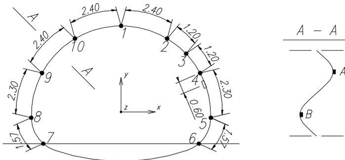
Fig. 3. Location of strain gauges
