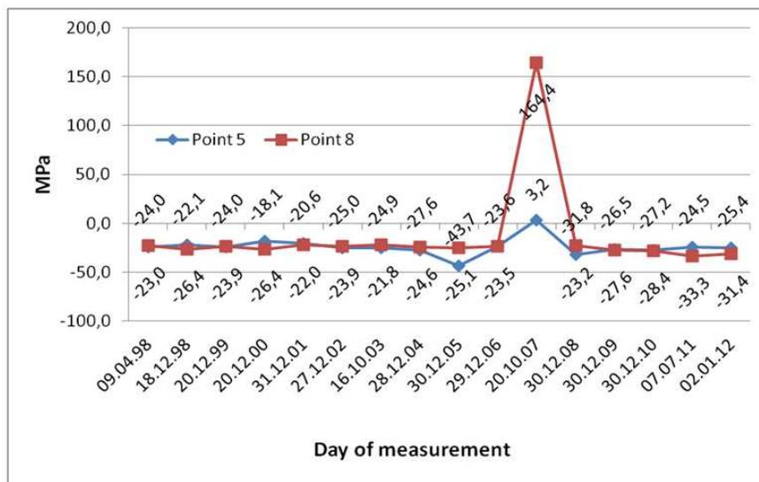
Fig. 12 Changes of hoop stresses in points 5 and 8 (near haunch)
