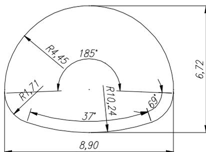
Fig. 2. Geometry of the tested structure
