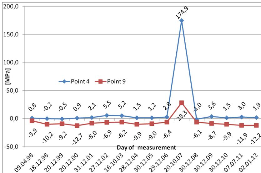
Fig. 10 Changes of hoop stresses in points 4 and 9 (side walls)
