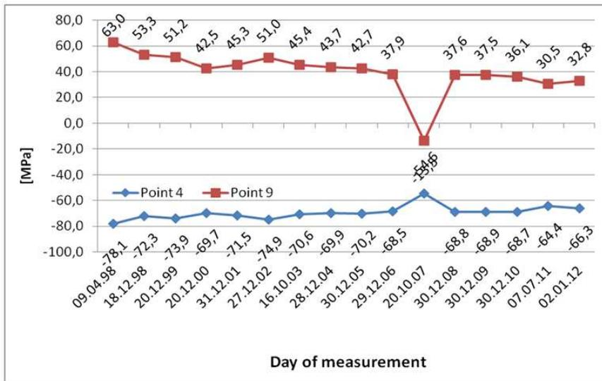
Fig.9 Changes of bending stresses in points 4 and 9 (side walls)
