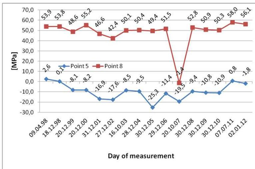
Fig. 11 Changes of bending stress in points 5 and 8 (haunch area )
