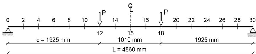
Fig. 5. Load scheme and section denotations in the element subjected to bending
