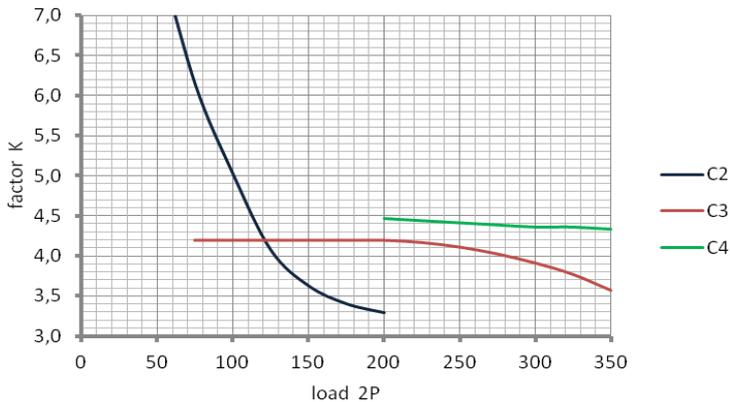
Fig. 6. Diagram of  $\kappa(P)$  function, specimen P1 (full cover plate)
