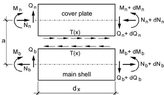
Fig. 3. Internal forces in a circumferential sector of a composite structure
