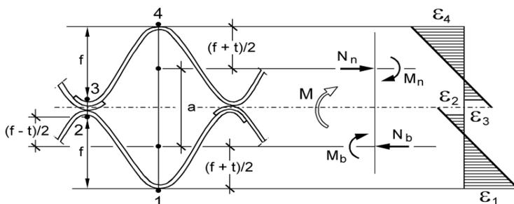
Fig. 2. Geometry, internal forces and strains in connected elements
