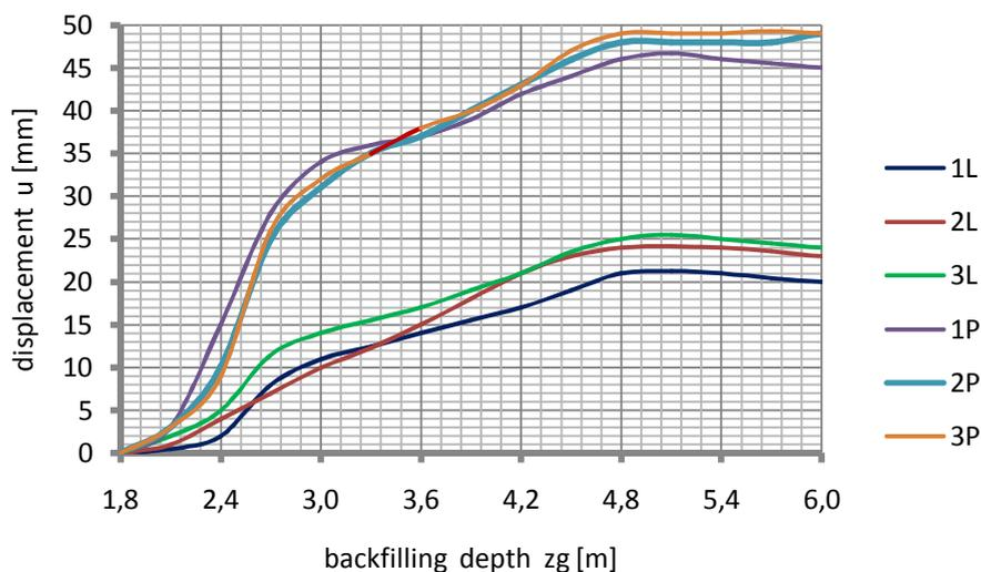
Fig. 3. Shell horizontal displacements (narrowing)
