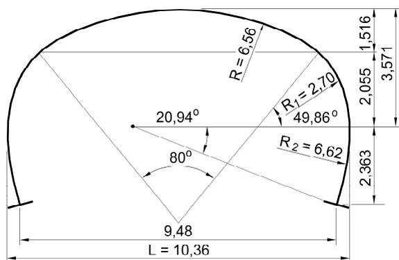
Fig. 2. Shell cross-section and geometry [m]
