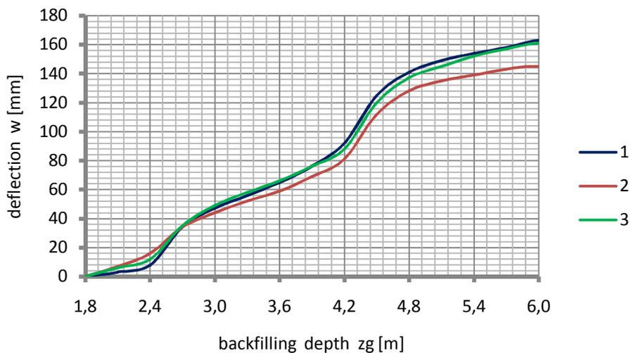
Fig. 4. Shell key course vertical displacements (uplift)
