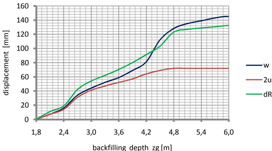
Fig. 5. Characteristic parameters of shell deformation
