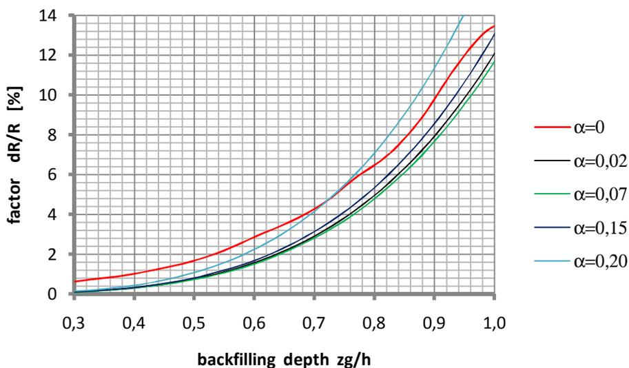
Fig. 7. Shell crown curvature changes during backfilling [5]
