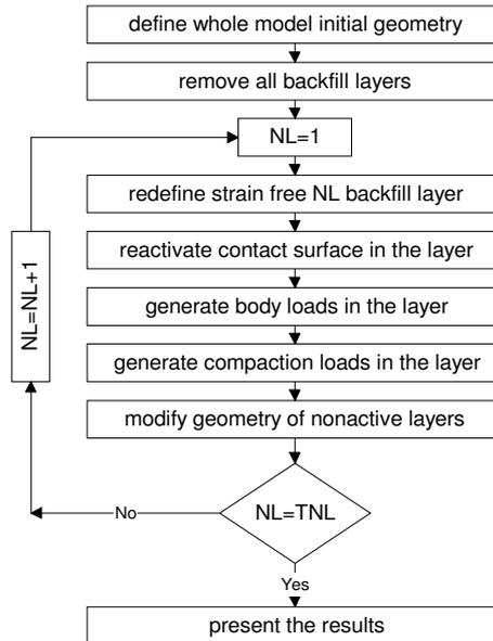
Figure 3. Flowchart of the procedure of construction process simulation. NL is a layer number, TNL is the total number of backfilling layers
