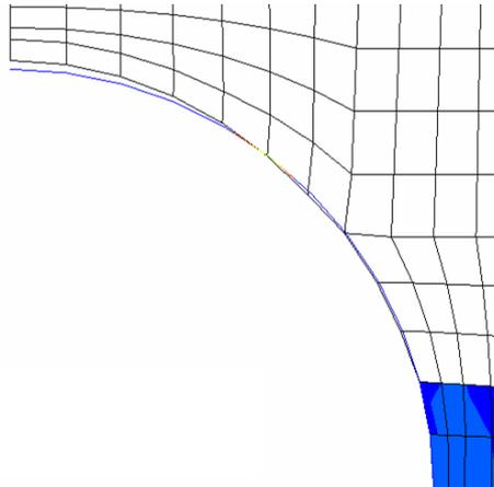
Figure 2. First layer reactivation. Inactive (white colour) elements present the final geometry configuration, unknown at this stage though
