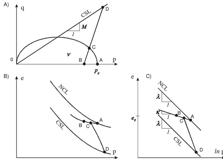
Figure 1. (A) Elliptical yield surface and critical state line (CSL); (B), (C) normal compression line (NCL) and unloading and recompression line; (0-A elastic-plastic hydrostatic compression, A-B elastic hydrostatic unloading, B-C elastic vertical loading, C-D elastic-plastic vertical loading of soil)
