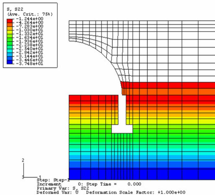
Figure 4. Finite element mesh and vertical stress distribution after generation of geostatic stress conditions and placement of the first backfill layer
