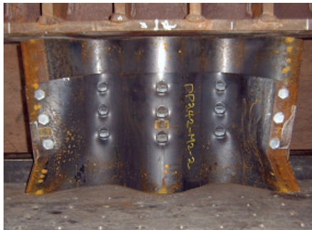
(a) t=6.23\text{mm} (SS490), bolt bearing
