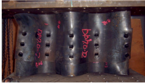
Fig 9. Failure of bolted seam with a F12.9T bolt for SS540 plate
