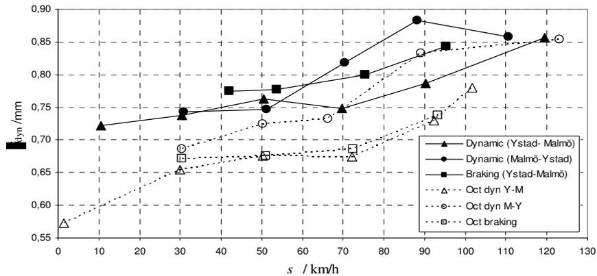
Figure 5. Maximum downwards vertical displacements of the crown during dynamic and braking tests
