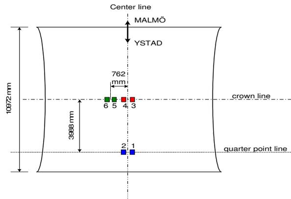
Figure 2. Culvert from the top with locations of strain gauges and travel directions
