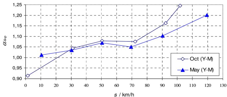
Figure 6. Dynamic amplification factors w.r.t. vertical displacements of the crown
