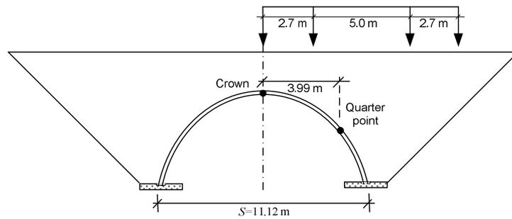
Figure 3. Demonstration of the static test axle loads when the first axle of the locomotive is above the crown of the culvert
