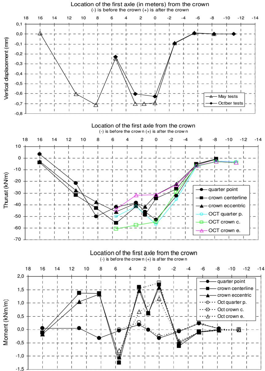
Figure 4. Maximum downwards vertical displacements of the crown, thrusts, and moments during static tests for different positions of the first axle of the locomotive
