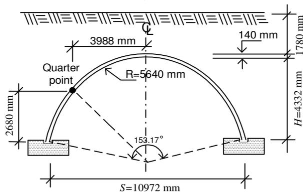
Figure 1. Sectional dimensions and geometry of the culvert structure (not to scale)
