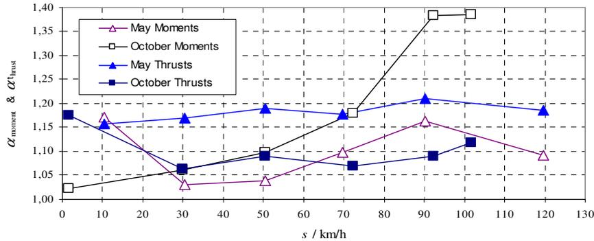
Figure 7. Average dynamic amplification factors w.r.t. moments and thrusts
