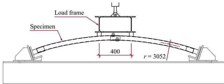
Figure 2. A sketch of the experimental setup. All dimensions are given in millimetres
