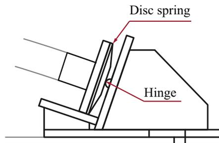
Figure 3. The support structure of the specimen
