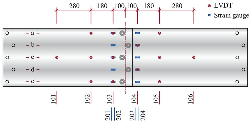
Figure 5. A schematic view of the instrumentation of the specimens. The displacement gauges (LVDT) were numbered 101 to 106. The strain gauges were numbered 201 to 204. The transversal location was indicated by the letters a to d
