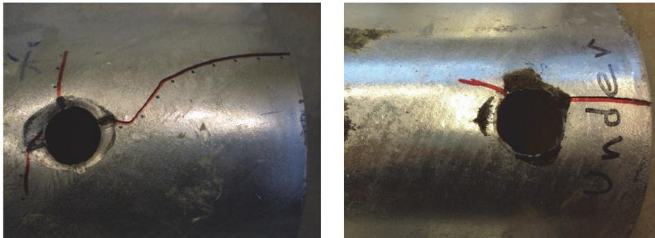
Figure 7. Crack patterns for specimen 1 and 6, respectively.
