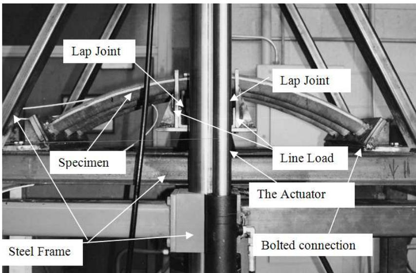
Figure 2: Lap Joint under Test and Loading Device
