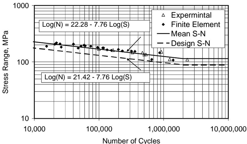
Figure 8: S-N Curve for Correct Lap Joint (No Misalignment)
