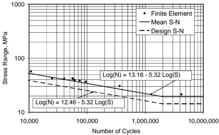
Figure 11: S-N Curve for Incorrect Lap Joint (4 mm Misalignment)
