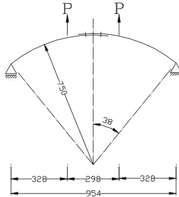
Figure 5: Model Dimensions and Statical System (All Dimensions are in mm)
