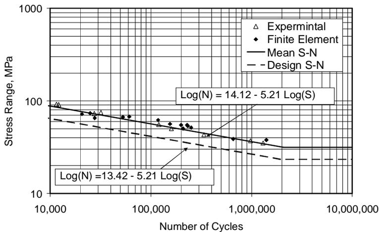
Figure 9: S-N Curve for Incorrect Lap Joint (No Misalignment)
