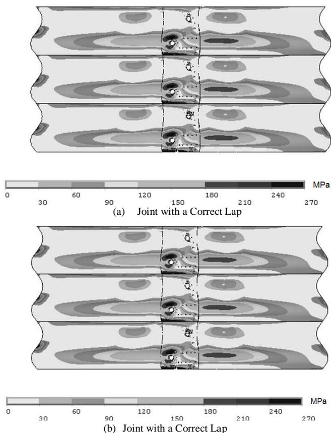
Figure 7: Stress Distribution in a Lap Joint
