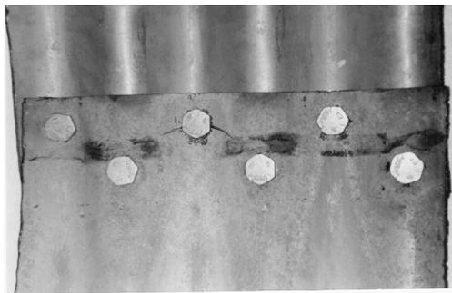
Figure 4: Observed Cracks in the Tested Joint (Correct Lap)
