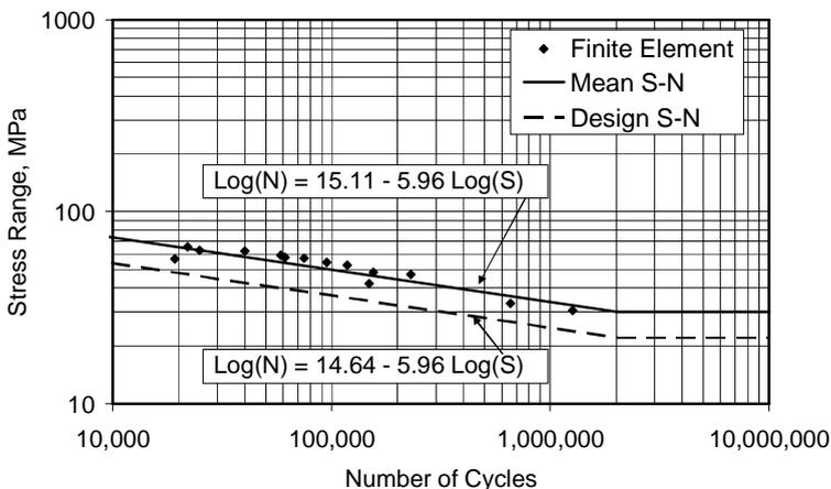
Figure 10: S-N Curve for Correct Lap Joint (4 mm Misalignment)
