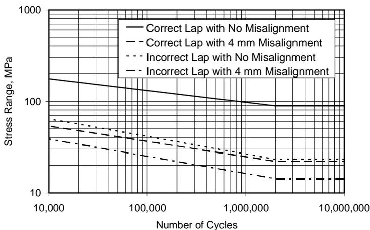
Figure 12: Comparison between S-N Curves for Different Lap Joints Configurations
