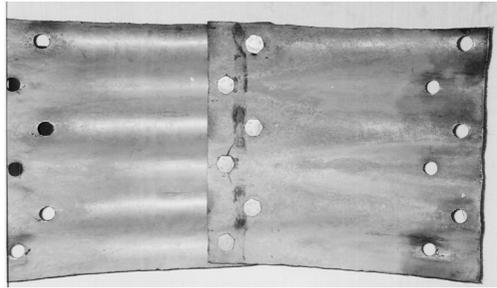
Figure 3: Top View of Tested Joint (Correct Lap)
