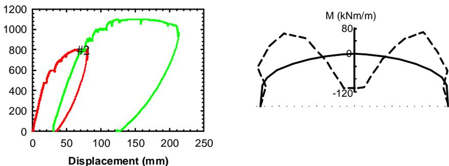
a. Load versus vertical deflection at the crown b. Moment distribution at peak load
