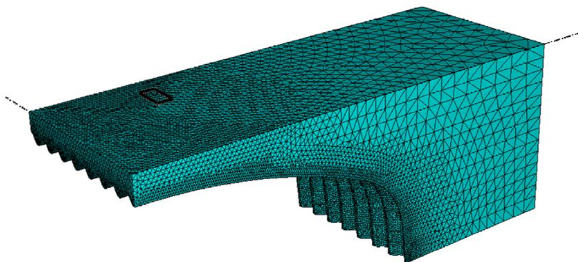
Figure 7. One quarter of the system modeled for the ultimate load test (Elshimi, 2011)
