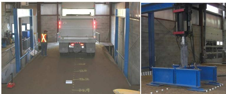
Figure 3. Loading with tandem axle dump truck and tandem axle loading frame
