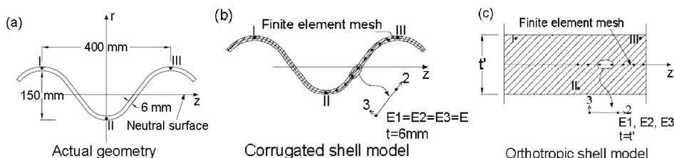
Figure 5. Corrugation geometry, 'corrugated shell' and 'orthotropic shell' models
