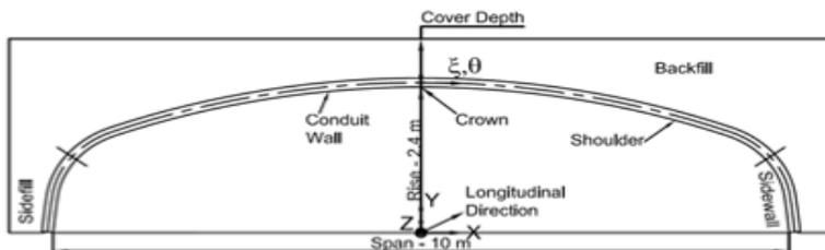
Figure 2. Cross-section of the large span box culvert (from Brachman et al. 2012)
