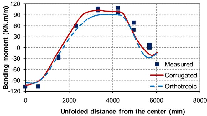
Figure 8. Moment distribution along centerline from crown to footing: calculated from measured strains and using ABAQUS at peak load (Elshimi, 2011)
