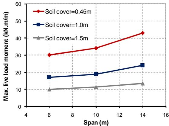
Figure 9. Peak bending moment due to surface load (from Elshimi, 2011)
