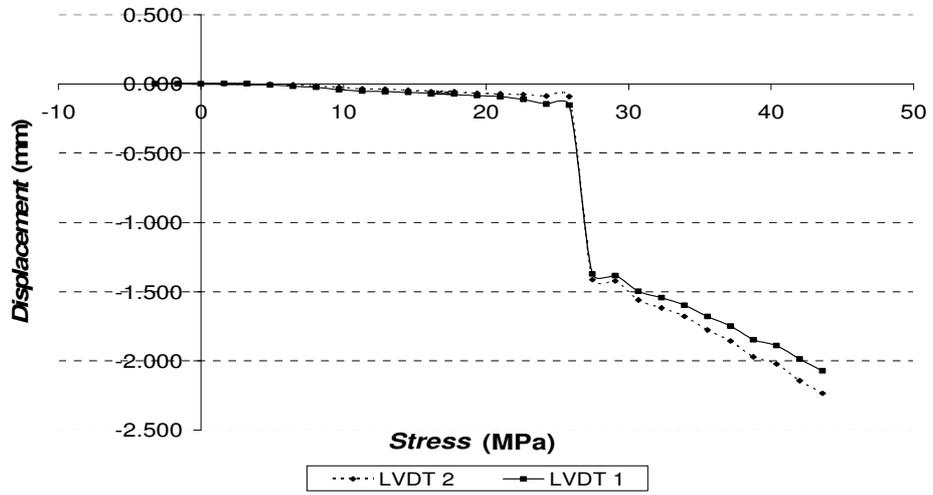
Figure 5. Stress vs. Displacement (237 N-m plates)
