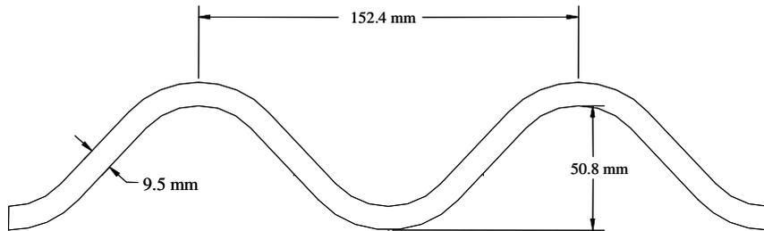
Figure 1. Profile View of Corrugated Steel Pipe
