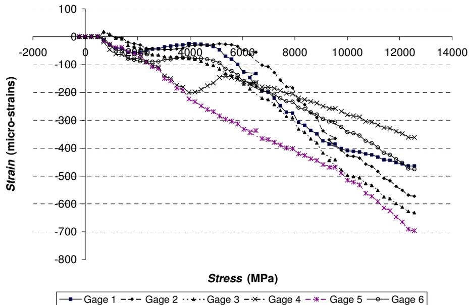
Figure 10. Stress vs. Strain (271 N-m plates)
