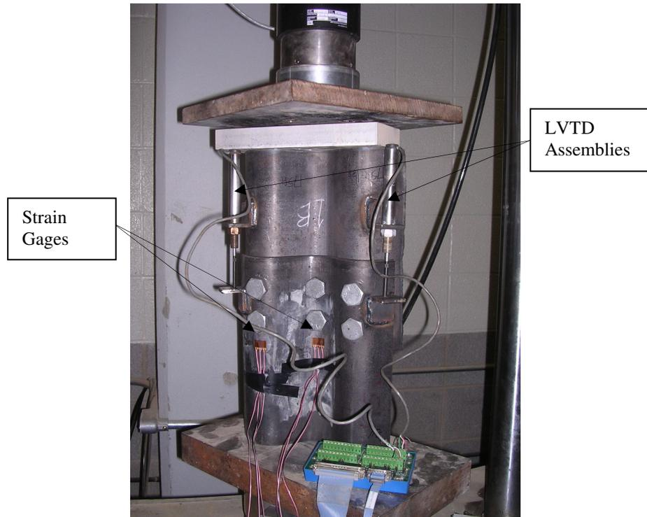
Figure 4. Testing of Instrumented Corrugated Plate Assembly
