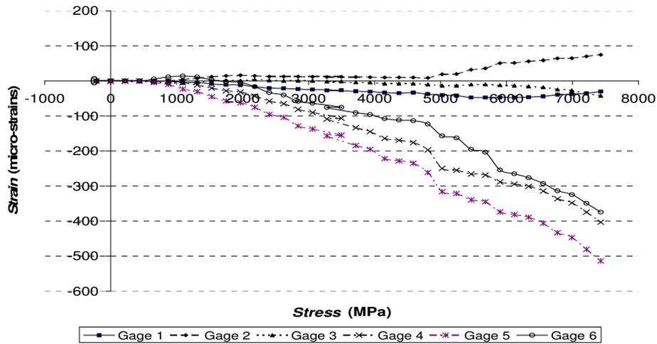
Figure 9. Stress vs. Strain (251 N-m plates)
