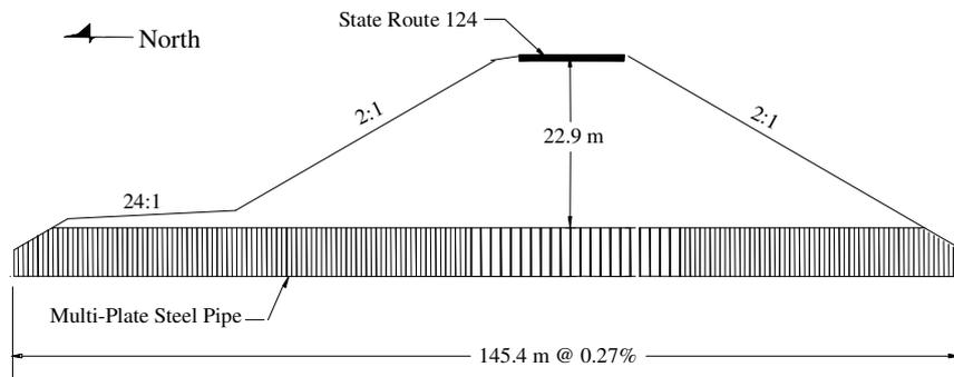
Figure 2. Profile View of Pipe Culvert Placed Under Embankment
