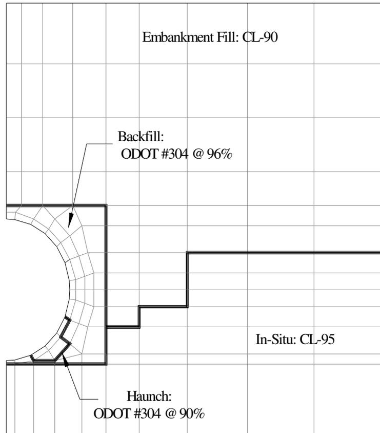
Figure 3. Half-Mesh Used in Numerical Simulation
