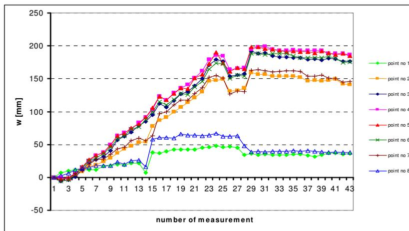
Figure 6. Change of deformations during construction
