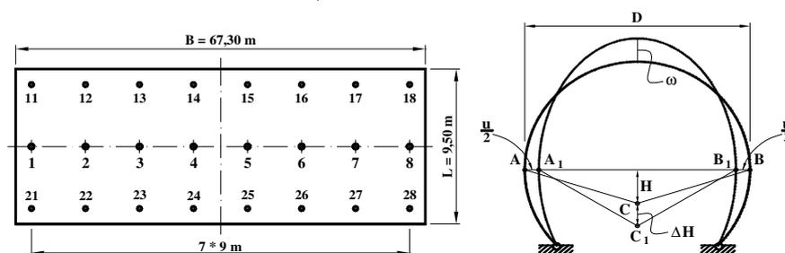
Figure 5. Location of measurement points in plane and way of measuring the deformations
