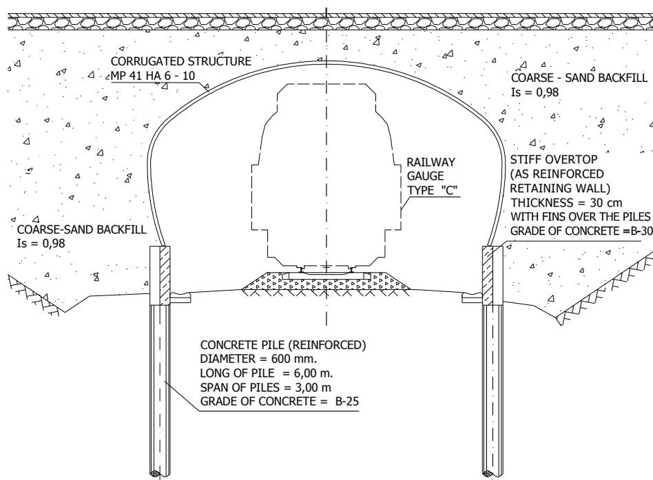
Figure 2. Cross section of the corrugated structure
