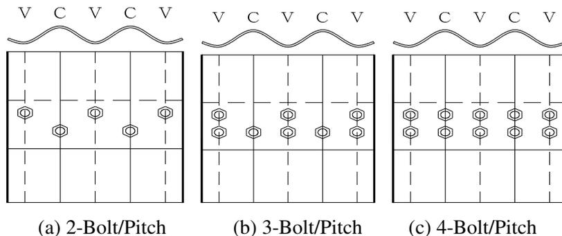
Figure 1. Standard bolt hole arrangement
