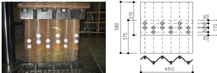
Figure 4. The View of the Compressing Test
