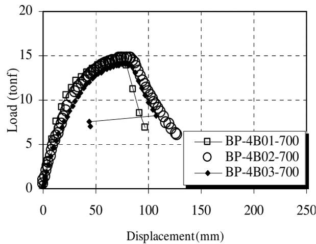
Figure 5. The result of the present 4-bolt seam
